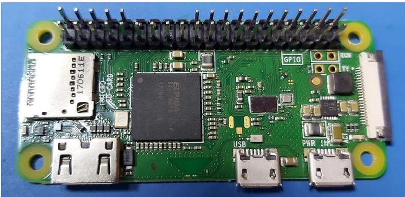
There are two versions of the Raspberry Pi Zero W and Raspberry Pi Zero WH. The “W” version does not come with headers and the “WH” version includes headers pre-soldered.
